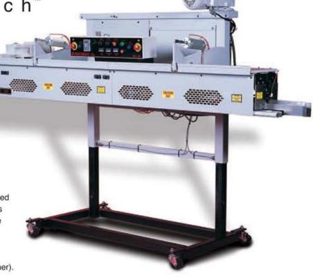
The PILS 300 is the ideal choice for closing a pinch-style bag with liners – the combination preferred when a controlled packaging environment and product sifting are concerns. The 300 first seals the bag's poly inner liner, then instantly reactivates the bag's pre-applied hot-melt adhesive strip and automatically folds over the top of the bag. The system securely controls the bag top throughout the closing process, ensuring a perfect, durable, sift-proof bag seal every time.
